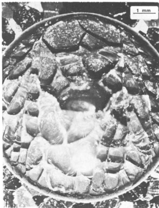
Figure 1 Base glass on Ti; test temperature T = 1100^\circ\text{C} . 2466
