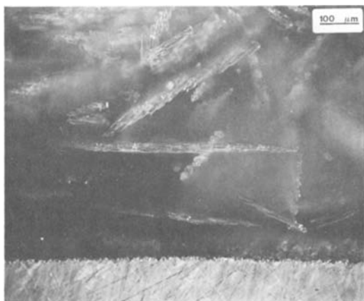
Figure 4 Crystals in 5% La-glass; polarized light; test temperature T = 1100^{\circ}C .
